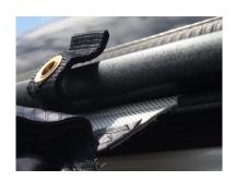
3. Peg down the rear pads at the back of the awning against the caravan using the adjustable pegging points. This keeps the awning in place whilst you inflate it. You may need to re-adjust them afterwards.
